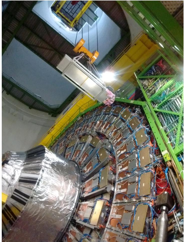
The CMS pixel detector was installed in 2017
